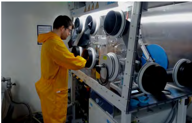
Figure 2: Christian Steyer loading uranium into the coating device inside the glovebox.
