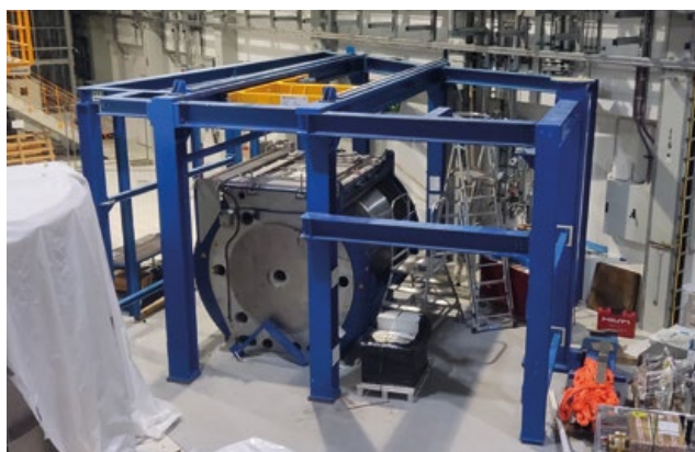
Figure 7: The sample chamber and the steel structure for the shielding house of POWTEX at its final position in the guide hall east.
